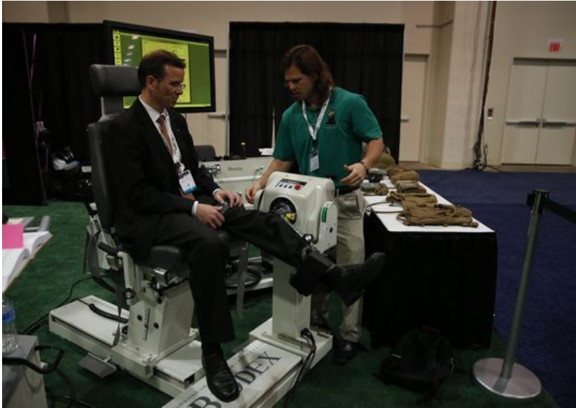
Justin Miller of Marine Corps Systems Command tests a subject's leg strength during the Navy League's Sea-Air-Space Exposition on April 15. The machine, typically used by professional sports teams, allows researchers to test the force required by Marines to complete various tasks. (Photo: Mike Morones/Staff)
