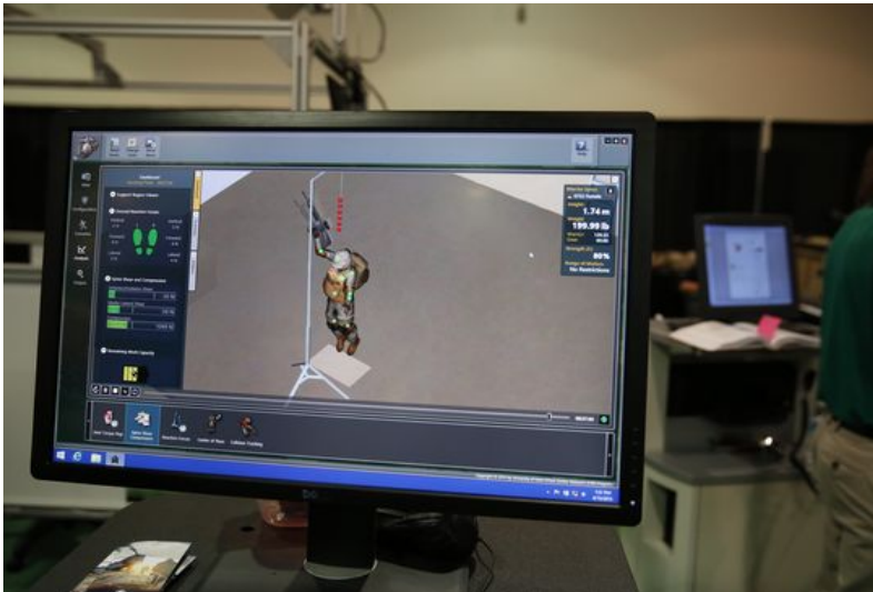
GruntSim, a computer simulation program, allows gear designers to outfit Marines with whichever pieces of kit they choose before running them through a virtual obstacle course that highlights joint stress. (Photo: Mike Morones/Staff)
