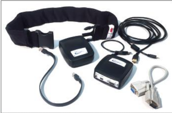
VibroTactile System; including tactile belt, linkbox, and cables.
