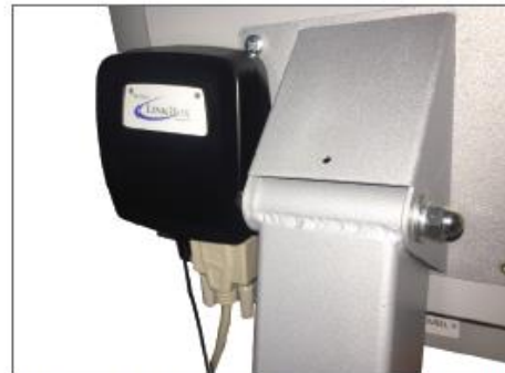
Linkbox wireless communication connected to the Biodex Balance System SD sends and receives signals from the tactile belt.
