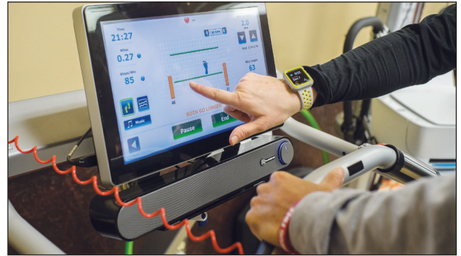
LCD screen on the Gait Trainer 3 provides visual guides for where each footfall should strike.
