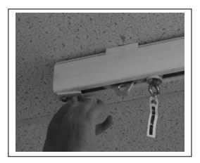
2. Place the harness clevis in the large eyelet. Note that the harness clevis connection contains a small hole in it. This is used to add a zip tie after the harness has been connected to prevent the clevis bolt from backing out.
