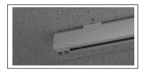
1. Remove the bumper with a ½-inch wrench. Place the Braking Trolley on the rail and re-install the bumper.
