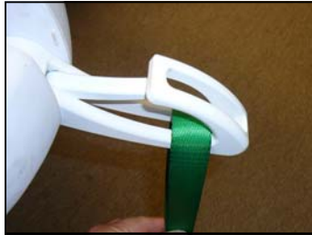
A) - Sling loop correctly positioned at the base of the P-600 carry bar hook.
