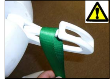
Figure 3 - Sling loop incorrectly resting on the P-600 hook locking clip.
