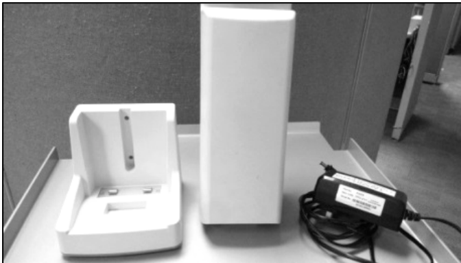
Figure 5-1. An optional stand-alone charging base allows a spare battery to be fully charged and ready for use at all times.
