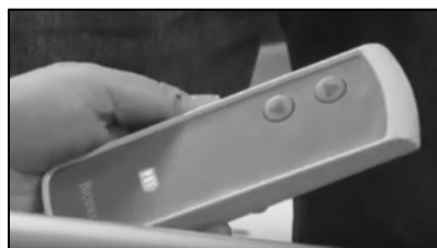
Figure 3-3. The Hand-Held Controller is used to easily raise or lower the Patient Cross Handle while assisting the patient to sit or stand.
