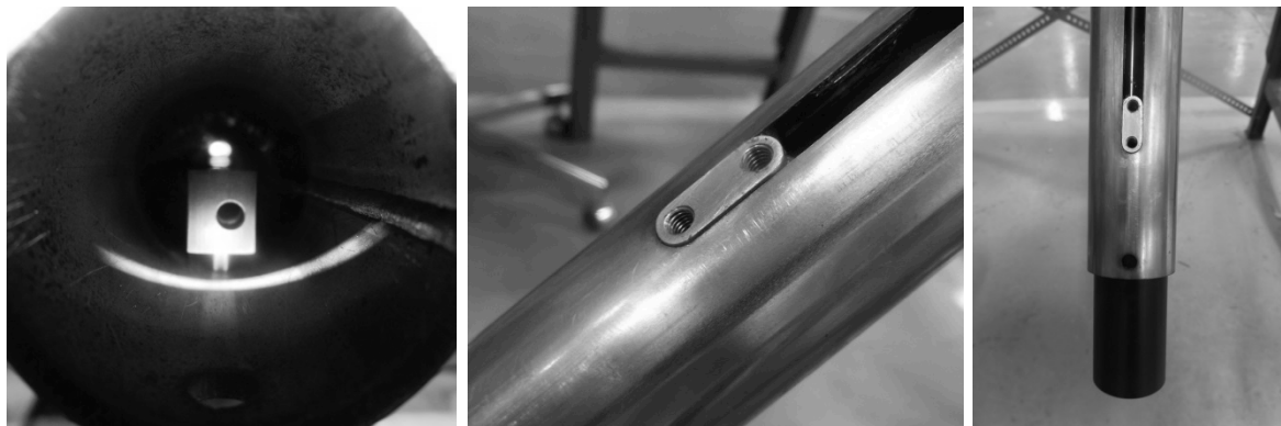
Figure 3.2. Mounting Block Engaged in Slot (Left), Mounting Block Flush in Slot (Center), and Male Tube Subassembly Shaft with Mounting Block Stopper (Right).
