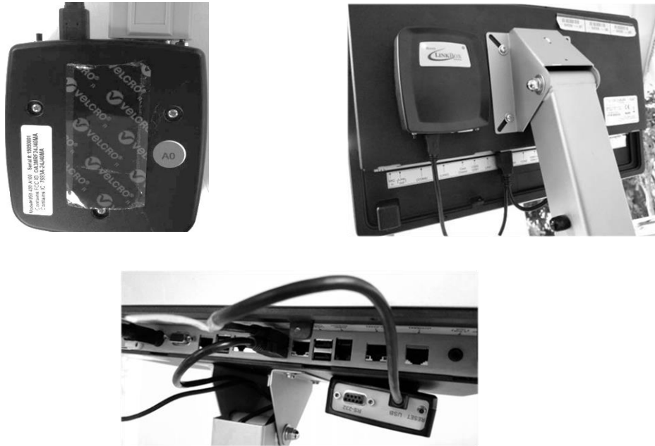
Figure 8.3. Installing the LinkBox to the Back of the Display.
