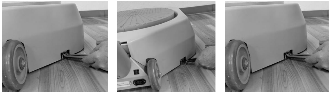
Figure 1.5 Leveling the Base.
