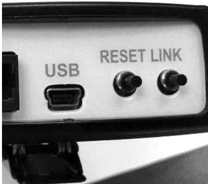
Figure 8.12. Touch LINK to Wireless Connect the Tactile Belt Receiver Box.
