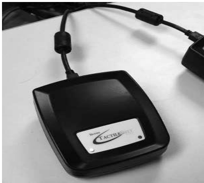
Figure 8.6. Tactile Belt Receiver Box LED Indicators.
