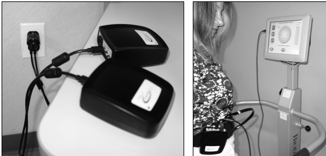
Figure 3.2 TactileBelt Receiver boxes can be charged with a connection to a wall outlet or to the display on the device.
