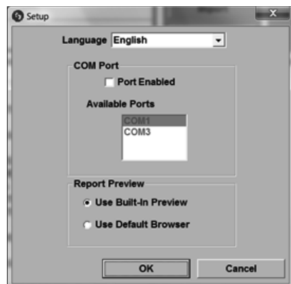
Figure 3.2. In the setup screen, select the desired language option and COM port if using serial connection for data transfer.
