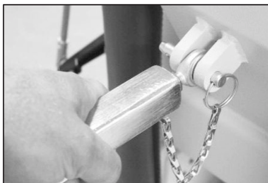
Figure 2.4. Attaching the Seat Back Brace to the System 4 Seat Back Clevis.
